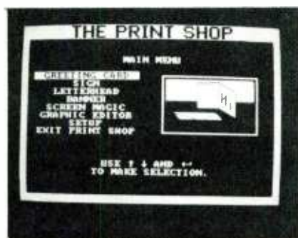
Fig. 2—Yes, it's really Print Shop on a TTL monochrome monitor (A). The usual all-graphics equipment display is shown in B. Notice the difference in how the text characters appear—the TTL display is somewhat smaller.
